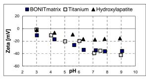
Fig.1: Comparison of Zeta potential measurements of BONITmatrix®, titanium and hydroxyapatite powder
